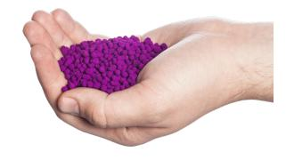
**Purafil SP Media** consists of generally spherical, porous pellets formed from a combination of activated alumina and other binders, suitably impregnated with sodium permanganate (NaMnO<sub>4</sub>). The sodium permanganate is applied during pellet formation such that it is uniformly distributed throughout the pellet volume and is completely available for reaction with target gases.
