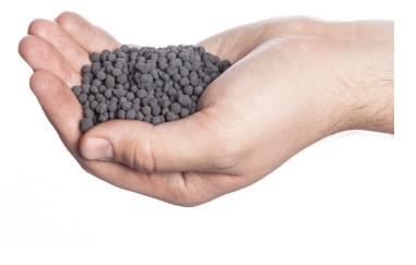
**Puracarb AM Media** consists of generally spherical, porous pellets formed from a combination of activated carbon, activated alumina and other binders, suitably impregnated to provide an enhanced removal capacity for ammonia and other basic (caustic) contaminants. Impregnants are applied during pellet formation such that they are uniformly distributed throughout the pellet volume and are completely available for reaction with target contaminants.
