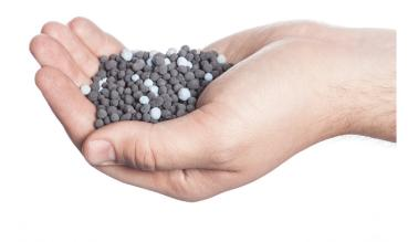
Odorcarb Ultra Media consists of generally spherical, porous pellets formed from a combination of activated carbon, activated alumina and other binders, suitably impregnated to provide a superior removal capacity for hydrogen sulfide (H<sub>2</sub>S). Impregnants are applied during pellet formation such that they are uniformly distributed throughout the pellet volume and are completely available for reaction with chlorine gas.
