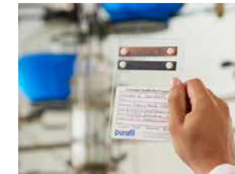
Purafil Corrosion Classification Coupon
