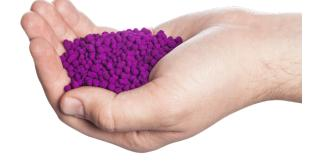
**Purafil SP Media** consists of generally spherical, porous pellets formed from a combination of activated alumina and other binders, suitably impregnated with sodium permanganate (NaMnO<sub>4</sub>). The sodium permanganate is applied during pellet formation such that it is uniformly distributed throughout the pellet volume and is completely available for reaction with target gases.
