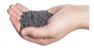
Puracarb Media consists of generally spherical, porous pellets formed from a combination of activated carbon, activated alumina and other binders, suitably impregnated to provide an enhanced removal capacity for acid gases and other corrosive contaminants in industrial environments. Impregnants are applied during pellet formation such that they are uniformly distributed throughout the pellet volume and are completely available for reaction with target gases.
