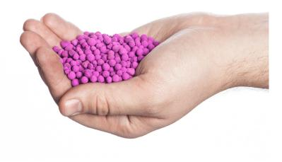
**Purafil Chemisorbant Media** consists of generally spherical, porous pellets formed from a combination of activated alumina and other binders, suitably impregnated with potassium permanganate (KMnO<sub>4</sub>). The potassium permanganate is applied during pellet formation such that it is uniformly distributed throughout the pellet volume and is completely available for reaction with target gases.
