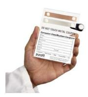
The Corrosion Classification Coupon + (CCC+) measures the amount of corrosion formation on copper and silver surfaces and logs the temperature and relative humidity of the immediate environment. This provides data allowing an industry standard classification of the amount of corrosion present as well as identifying contaminant classes.
