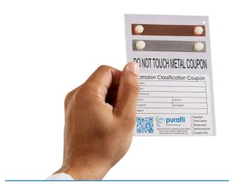
the type and thickness of corrosion films on the surface of each metal coupon. A normalized 30-day reactivity rate is calculated using the amount of time the metal coupon is exposed and the thickness of the corrosion that has formed.
