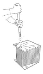
5. Open the media sampling probe and insert the device into the module via the sampling port. Once media has filled the device's lower portion, close the probe and remove it from the module.
