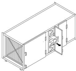
4. Set the module up on its end so that the sampling port faces up and remove the plug from the sampling port.
