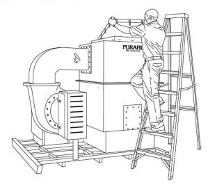
4. To take a sample, first open your media sampling probe. Insert the probe into the unit until the open portion of the probe is approximately 6 inches from the top of the unit. Once media has filled the device's lower portion, close the probe and remove it from the unit.
