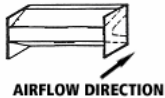
Figure 3: Module Position for Installation Into Vertical Unit Direction of Installation
