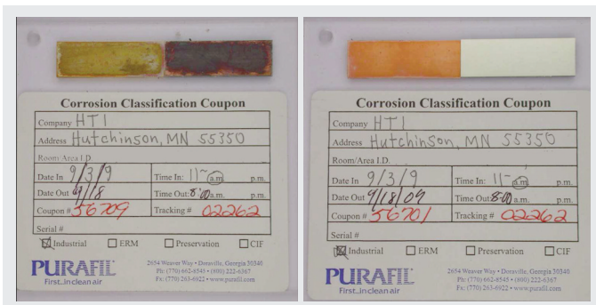
Purafil® Corrosion Classification Coupon placed upstream depicts a Severe or GX Environment
